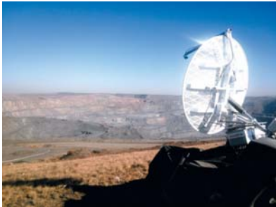
Slope stability radar at Inner Mongolia Pacific
