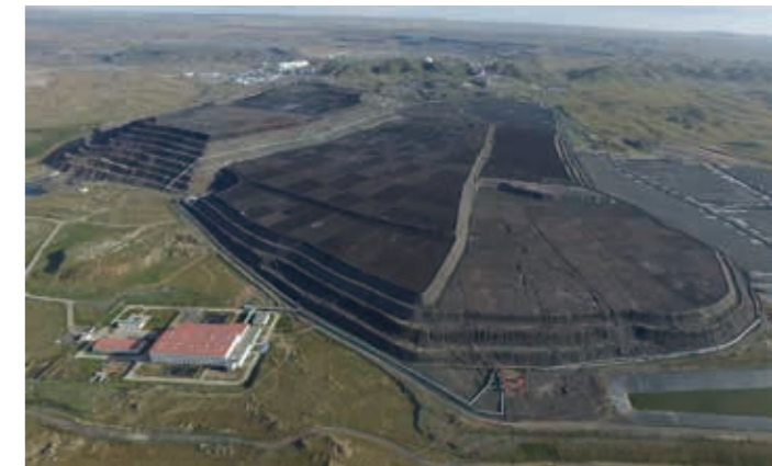
CSH Mine's heap leaching field
