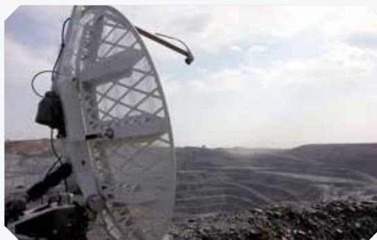
Slope radar at open mine of CSH Mine
