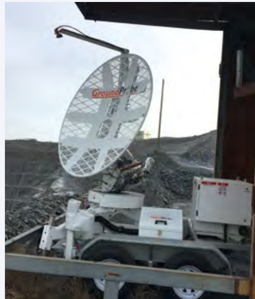
Slope monitoring radar of open-pit of the CSH Mine
