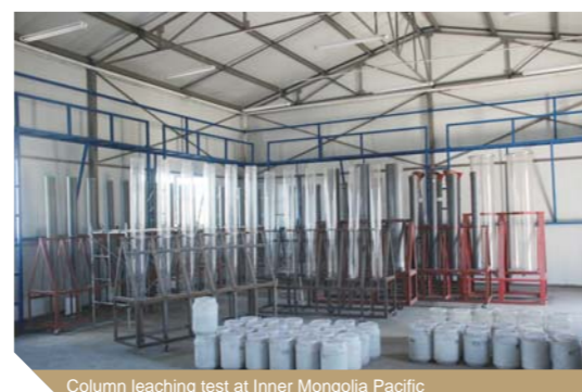
Column leaching test at Inner Mongolia Pacific
